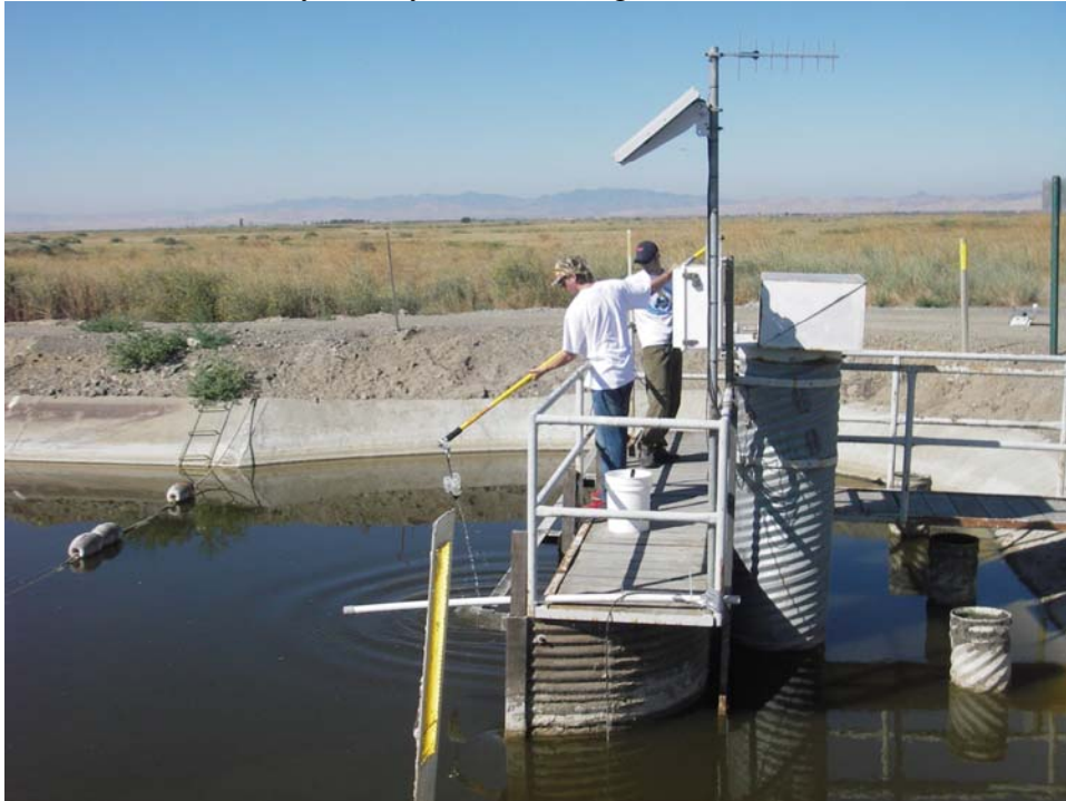
Figure 24: Depth integrated sampling at DO-44, San Luis Drain End. The pole and bottle holder are designed to fill bottles slowly as they decent through the water column.
