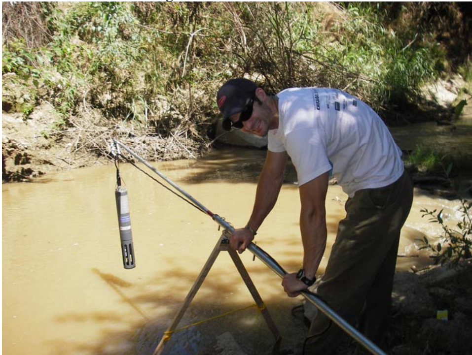
Figure 25: In-situ measurement of chlorophyll-a and other water quality parameters using a YSI 6600 sonde at DO-21, Orestimba Creek. The tripod allows the sonde to be placed further into the middle of the flow without wading.
