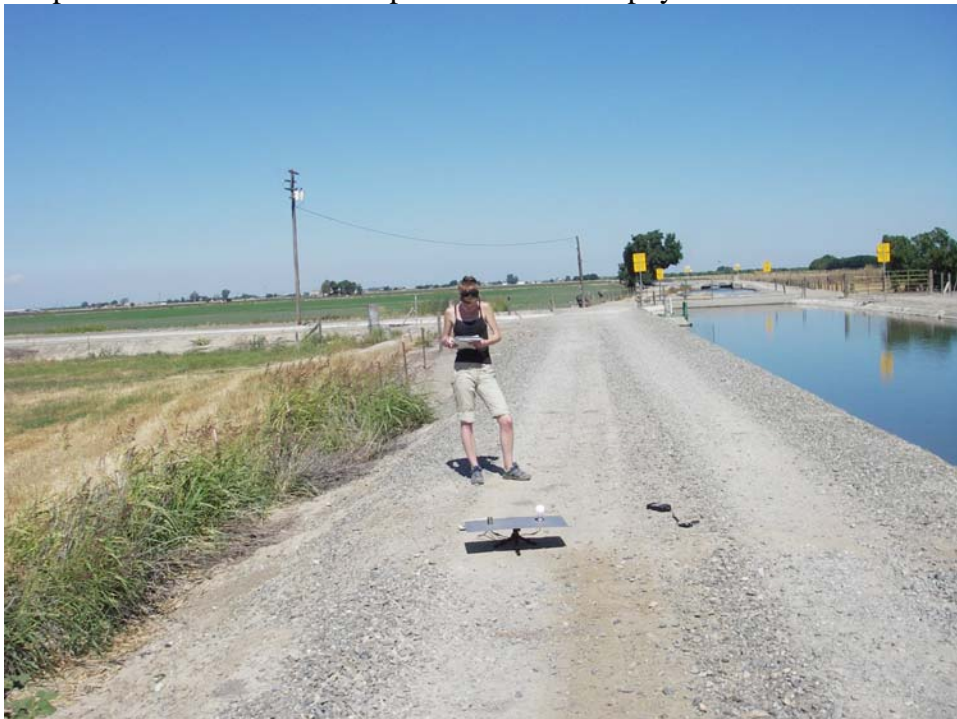
Figure 27: Measurement of incident light with spherical and flat quantum light detectors. Light is measured to provide reference for interpretation of chlorophyll-a results.
