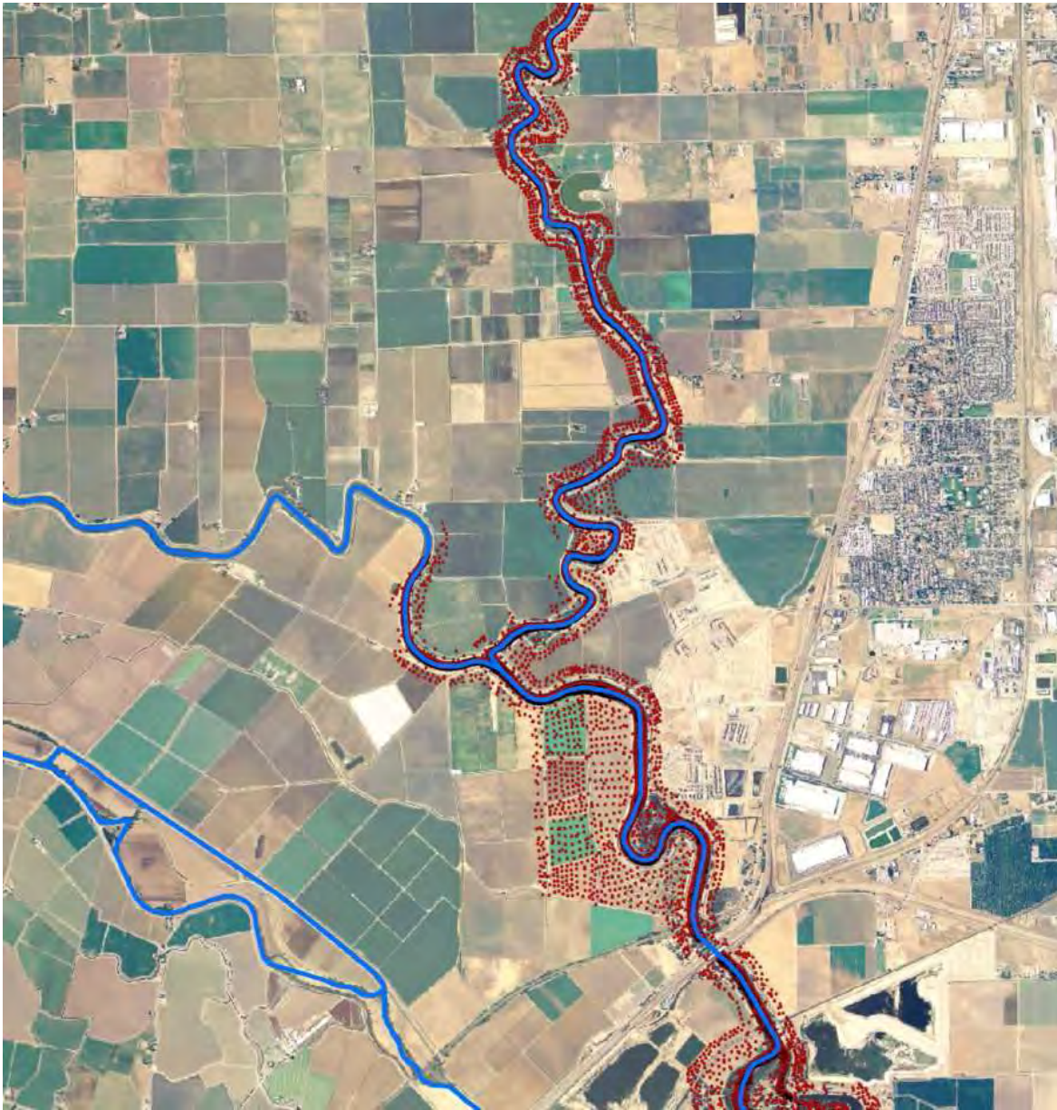
Figure 2. Model reach showing the US Corps of Engineers channel cross-section and DEM dataset that was made available through a US Bureau of Reclamation – Department of Water Resources cooperative agreement. Data is of sufficient refinement to allow accurate 3-D cross section profiles to be developed for the model study reach between the Vernalis and Rough and Ready Island monitoring stations.
