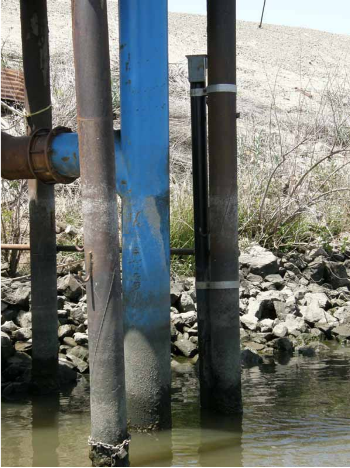
Figure A-15: The permanent 4" ABS pipe sonde housing installed at SBC.
