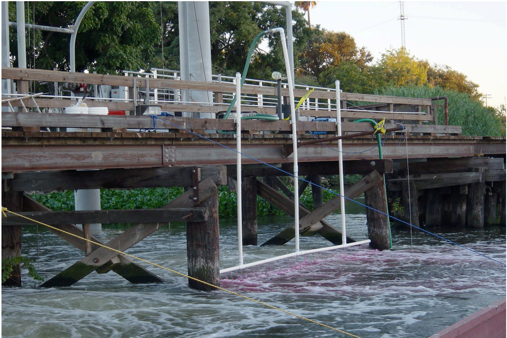
Figure 2: Rhodamine WT tracer injection into Port of Stockton aerator upwelling bubble flow.
