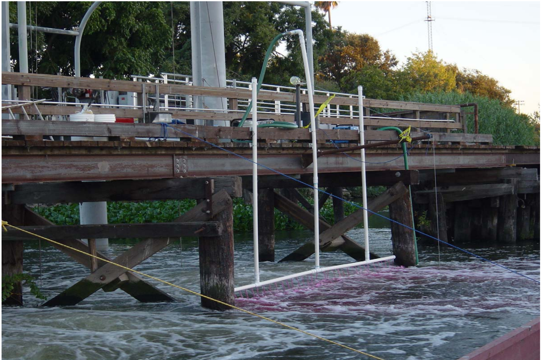
Figure 9: Rhodamine WT tracer injection into Port of Stockton aerator upwelling bubble flow.
