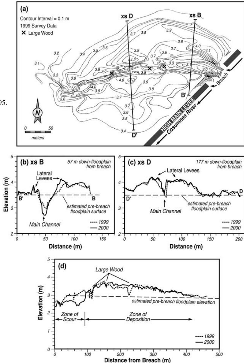
establishment and growth of riparian vegetation. Based on field surveys of lateral levee elevations and high water marks, we estimate that the maximum height of accretion in lateral levees is approximately .4 the maximum depth of local flow. For this reason, the elevation and morphology of the lateral levees is strongly controlled by the maximum flood stage recorded since the opening of the breach.
