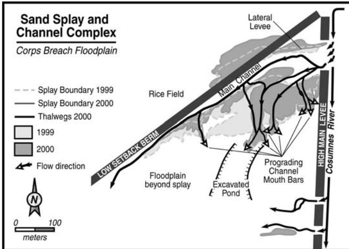
FIGURE 2. Generalized geomorphic map of the Corps Breach constructed during Fall of 1997. Note complex topography and growth patterns of sand splay complex due to set back levee (from Florsheim and Mount, in press).
