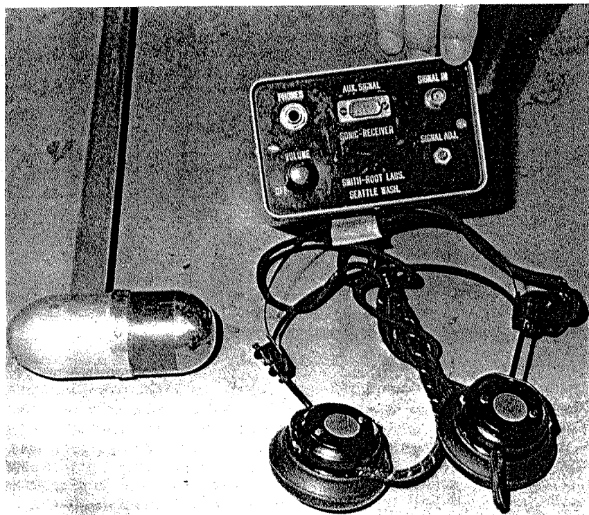
FIGURE 8. Portable probe (or hydrophone) and receiver for tracking sonic tags. Photograph by John A. Shaver.
