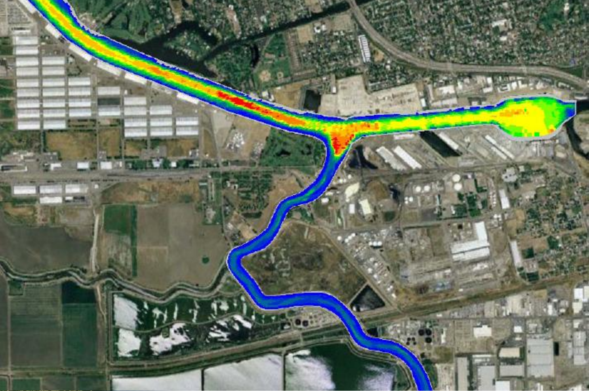
Bathymetry map of San Joaquin River channel at point of entry to the Deep Water Ship Canal
